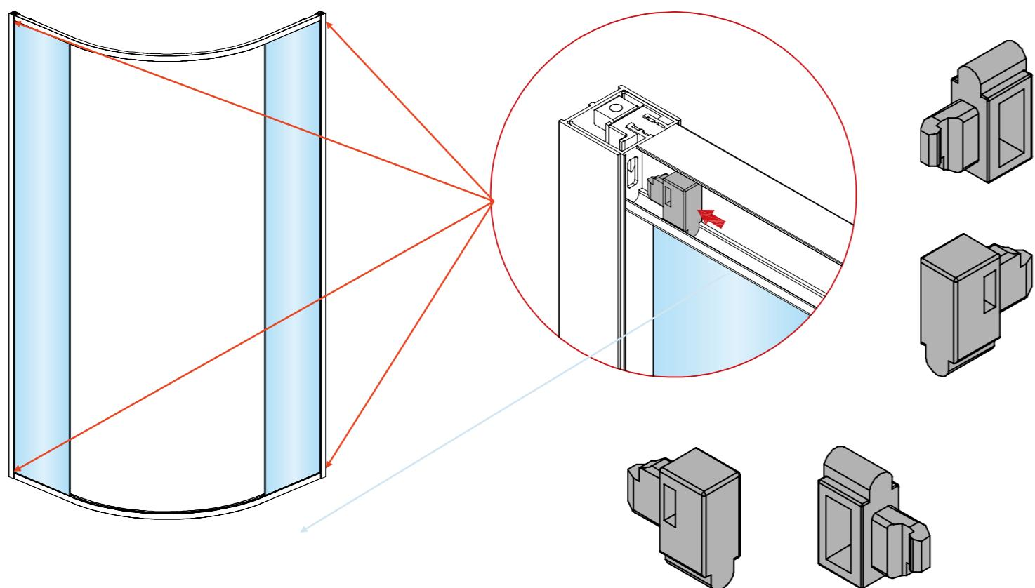
Insert the nylon part to the notch of the vertical profile, the notch will catch the nylon part and then hard to come out without tools.
